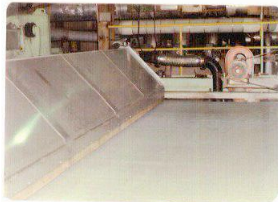
#26 / #27 – Non-profiling Lazy Steam Hoods are very simple in design
