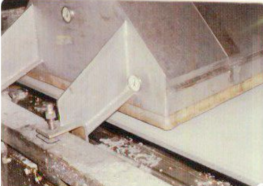
#24 / #25 – Non-profiling Lazy Steam Hoods for uniform steam application
