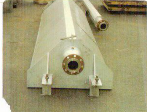
#24 / #25 – Non-profiling Lazy Steam Hoods for uniform steam application
