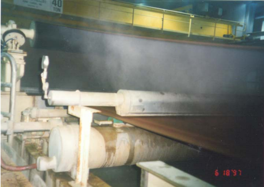
Figure 6 – Non-turbulent steam shower centered 1" above top fabric uhle box
